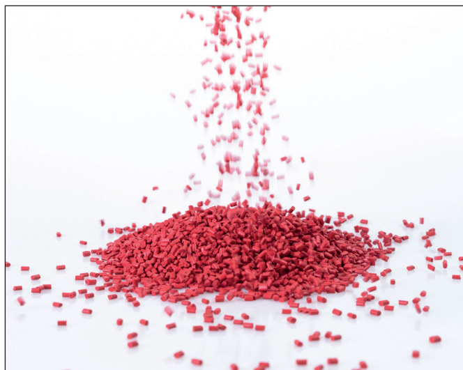
Fig. 2: Plastic granulate for injection molding or extrusion
