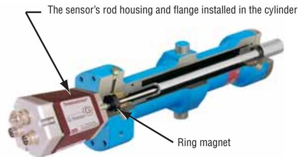
Figure 9. Fluid cylinder installation example
