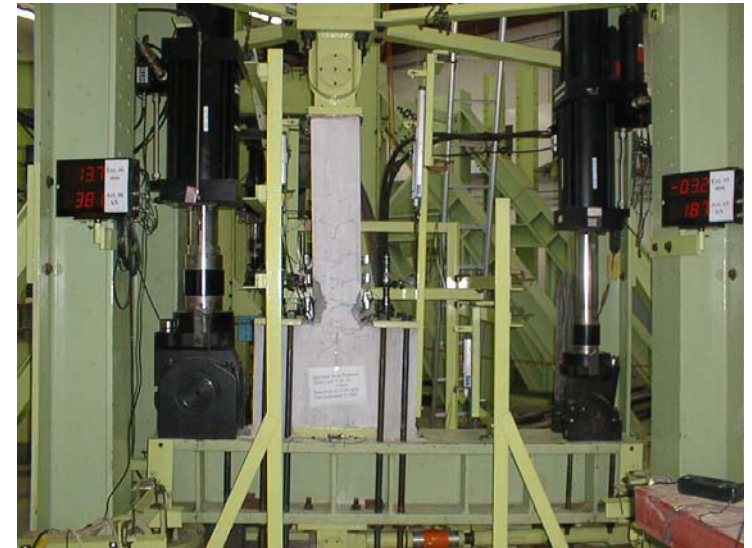
Destructive Test Measurement, (10 x LP / analog)
